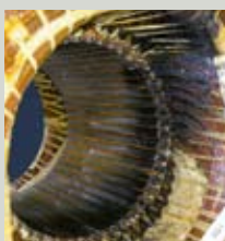
High level of oil acidity Corrosion on the motor windings resulting in motor burn out
