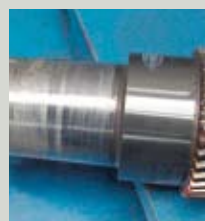
Components wear High wear on bearing causing compressor failure
