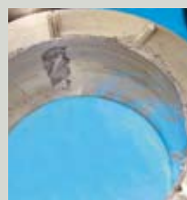
Components wear High wear on bearing causing compressor failure
