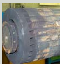
High level of oil acidity Corrosion on the motor windings resulting in motor burn out
