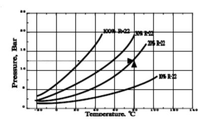
3. In order to determine the viscosity of the mixture, the 20% dilution is paired with the oil supply temperature to obtain the mixture viscosity. For example, if the oil supply temperature was 122°F (50°C), the dilution is 20% from above, the resulting mixture viscosity would be approximately 28-29 cSt. The chart on the following page outlines the process:
