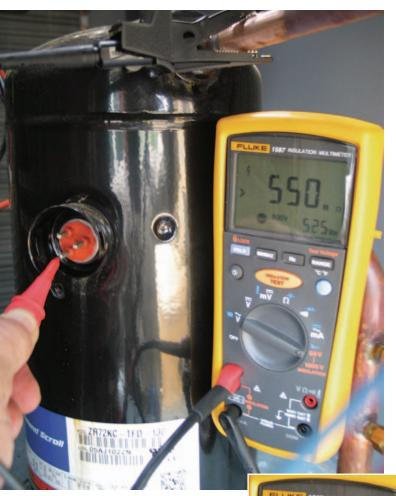
At an applied voltage of 500V, this IRT reading shows >550 M $\Omega$ , indicating resistance is out of range. A second IR test was performed at 1000 V and showed 1.1 G $\Omega$  (1100 M $\Omega$ ). If no leakage current had been detected, a reading would have been >2.2 G $\Omega$ . The Fluke 1587 insulation multimeter combines the features of a DMM (volts, ohms, millivolts, milliamps, frequency, capacitance, temperature) with a megohm meter for comprehensive motor maintenance.
